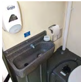
Toilet wash area The onboard heating system delivers warm water to the forearm wash basin in the toilet area.
